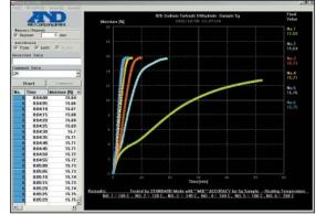
RsFig measuring the Sodium Tartrate standard provided with all analyzers. Graph demonstrates excellent repeatability as moisture values converge when tested at different temperatures.
