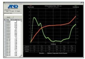
RsTemp function tracks % moisture (red) and drying rate (green) vs. time. Here coffee is measured.
