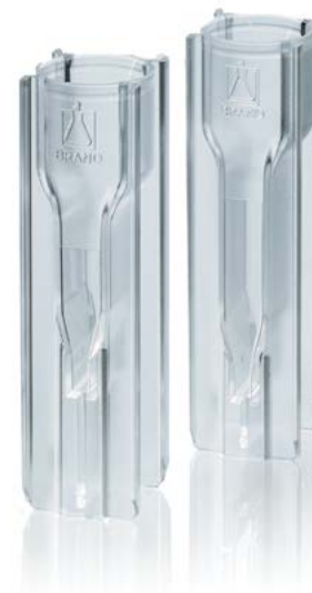
BRAND® ultra-micro UV-Cuvettes. 15 mm (left) and 8.5 mm (right) window heights
